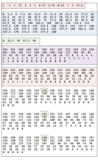
Following the metadata is the series of vertical angles in the photometric web. This file contains data for all of these 73 vertical angles.
