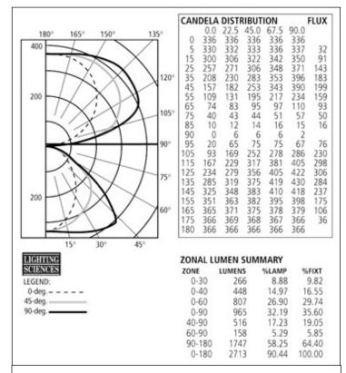
Example of a direct/indirect, bilaterally symmetric photometric distribution.
